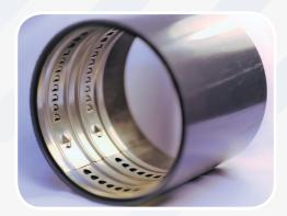
CUES-Lock End Sealers are used to seal the annular space between the cured-in-place liner and the host pipe at the pipe ends. It prevents the ends of the cured-in-place liner from delaminating or sagging from the host pipe.
