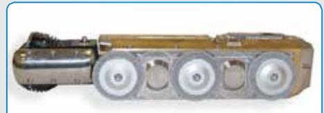
CPR in the 6" Steel Configuration
