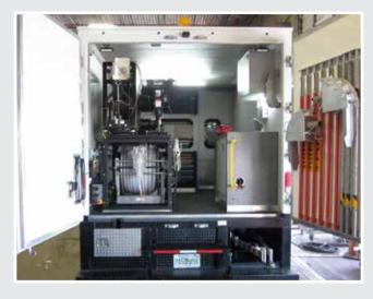
Custom CCTV/Cutter Truck and Trailermounted units include full capabilities for reinstating lateral services, removal of protruding taps, brush finishing existing cuts, and pre and post TV inspection.
