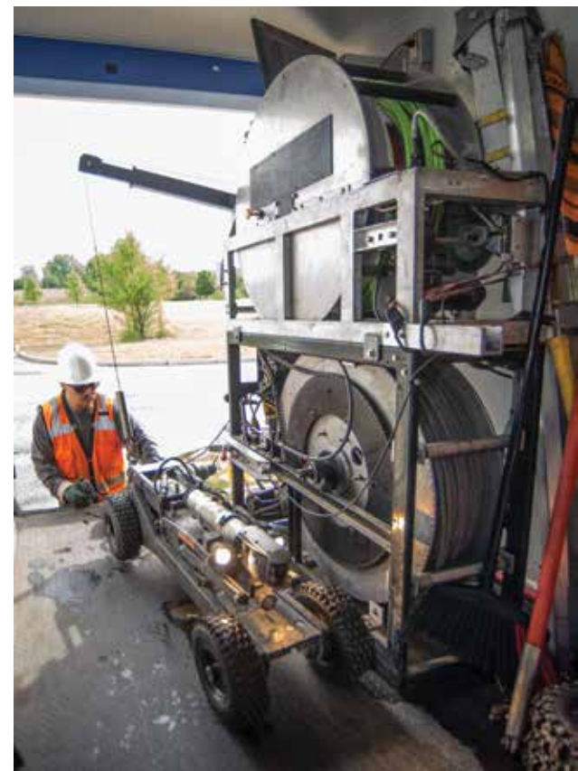
ABOVE: TREKK technician Gabe Gonzalez runs a sewer inspection from the control room of a CUES inspection van. BELOW: Gonzalez uses a winch to get the CUES Mud Master camera out of the CCTV van at the start of an inspection job.
