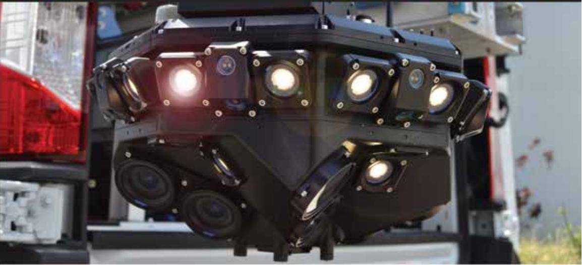
The CUES SPiDER Scanner is the first wireless and color manhole inspection technology of its kind, built in a lightweight and compact form factor.
