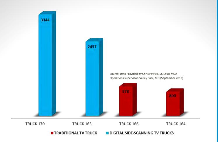
The two digital side-scanning trucks outperformed the traditional CCTV systems by 4,023 feet. Essentially, the digital side-scanning trucks were 3x more productive in the same working day than that of their traditional counterparts.
