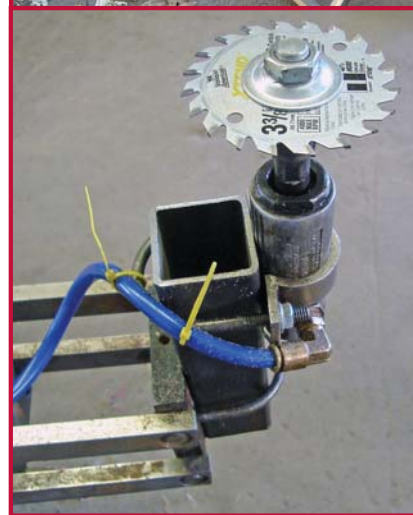
The 3.5-inch blade is mounted on the high-speed air cutter motor.
