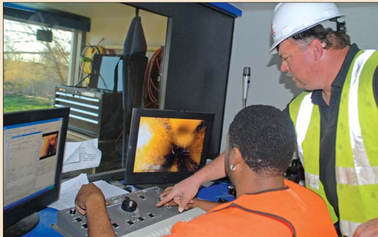
Technicians Bruce Walter and Paul Bordelon check video images in a camera truck. The camera collects data on runs up to 700 feet long.
