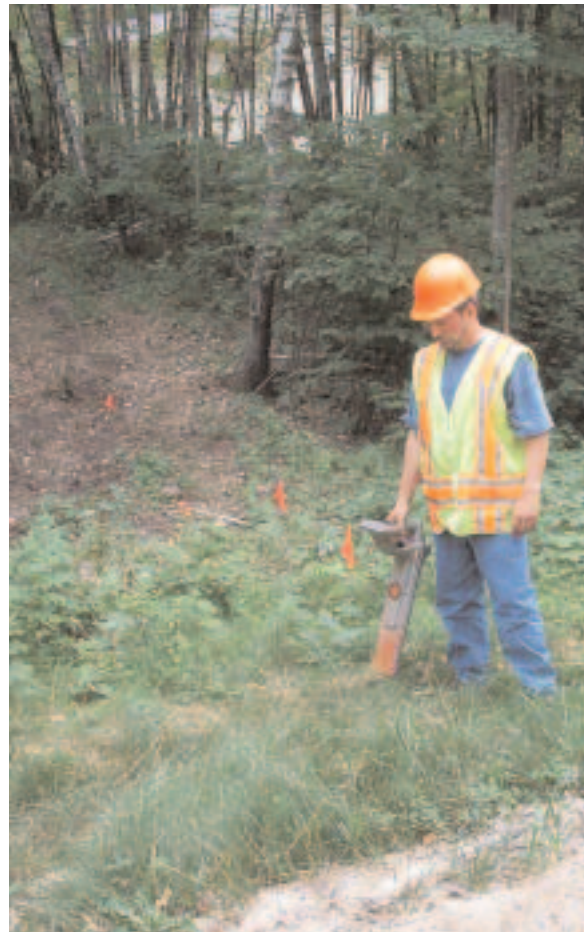
Locator Erik Lawson uses a Radiodetection RD400 Line Locating unit while marking utilities for Citi Lites, Inc., a 15-year-old, family-run locating business that provides statewide coverage from its base in Pequot Lakes, Minn. (218-568-4744).
